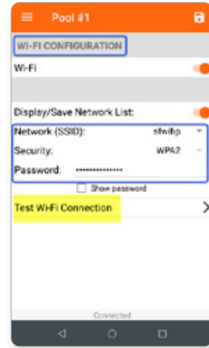
Fig. 10.17: Test Wi-Fi Connection
